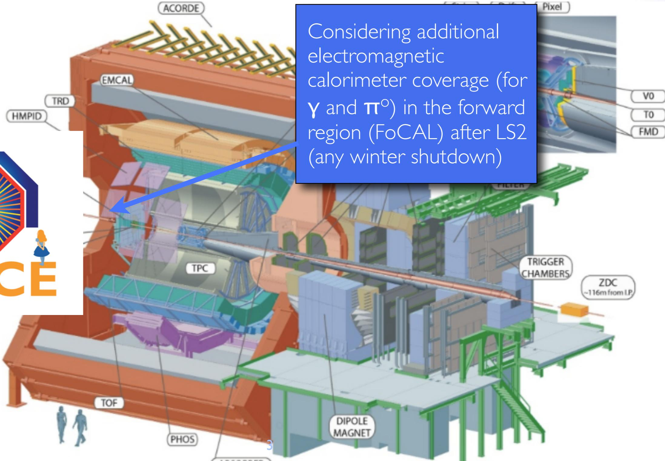
Considering additional electromagnetic calorimeter coverage (for  $\gamma$  and  $\pi^0$ ) in the forward region (FoCAL) after LS2 (any winter shutdown)
