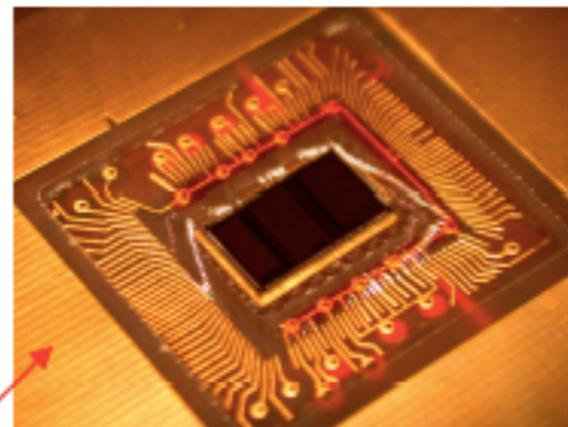
Chip embedded and encapsulated
