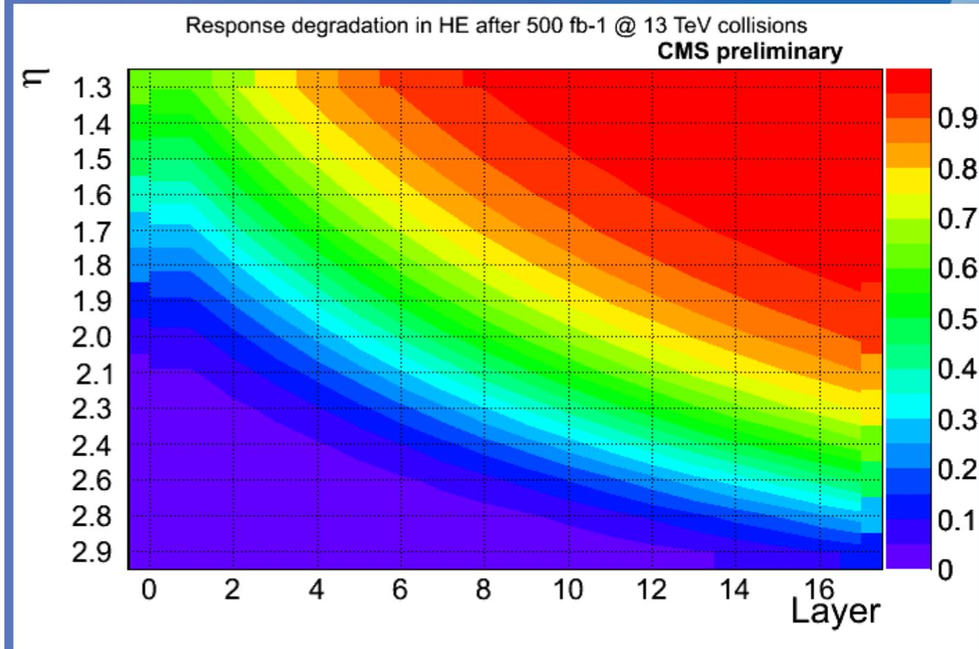
In the endcap radiation damage is very severe. It will require upgrade of the endcap ECAL+HCAL detector before HL-LHC
