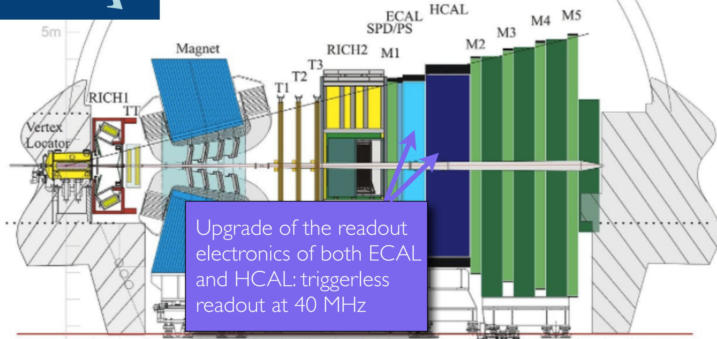
Upgrade of the readout electronics of both ECAL and HCAL: triggerless readout at 40 MHz
