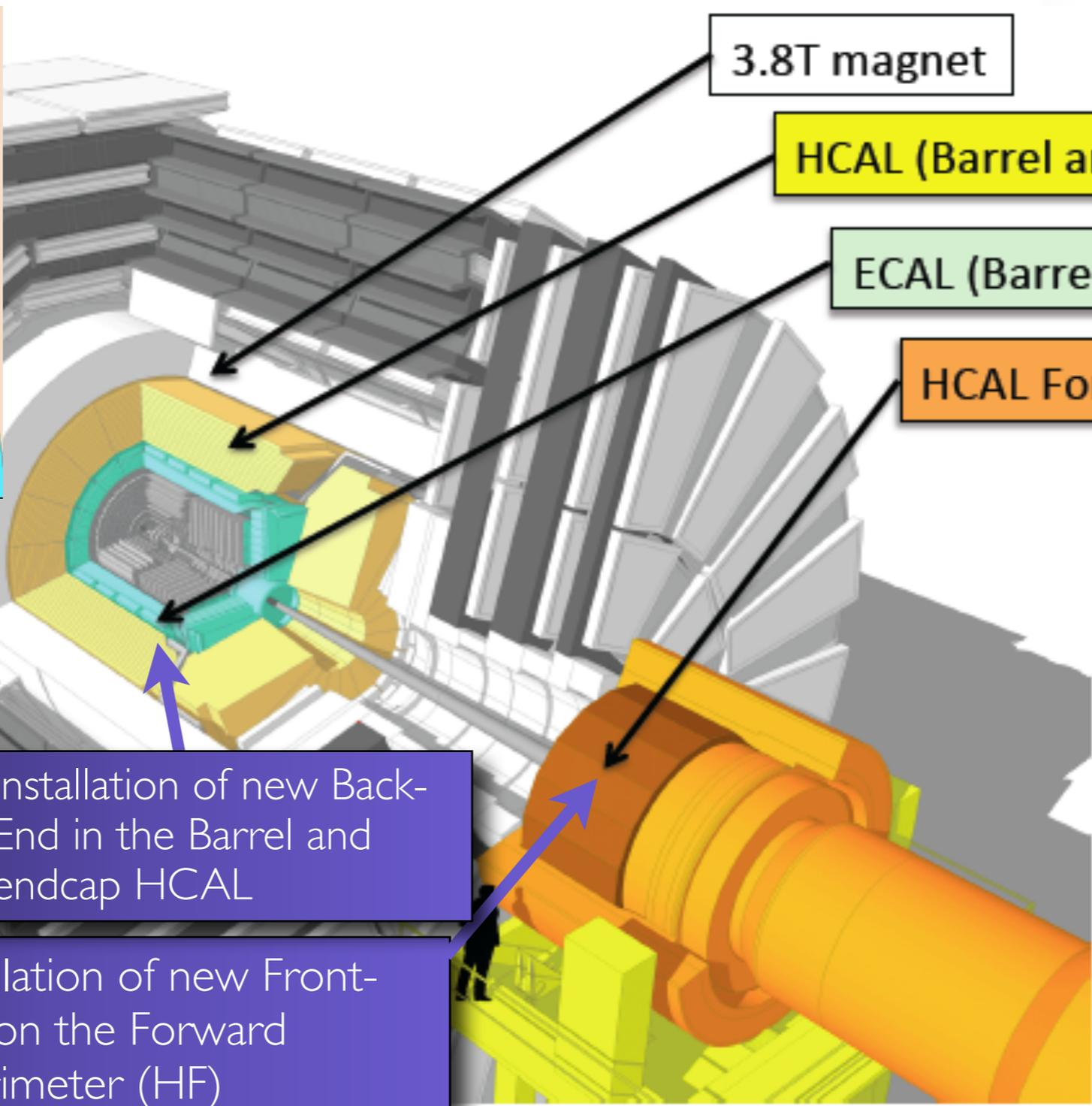
Installation of new Back-End in the Barrel and endcap HCAL
