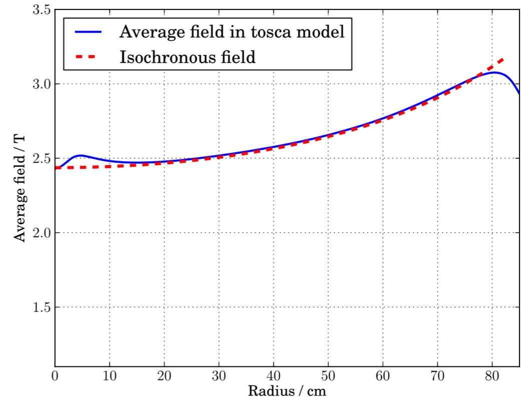
Average field with initial isochronous shaping; iterative process by evaluating tosca models.
