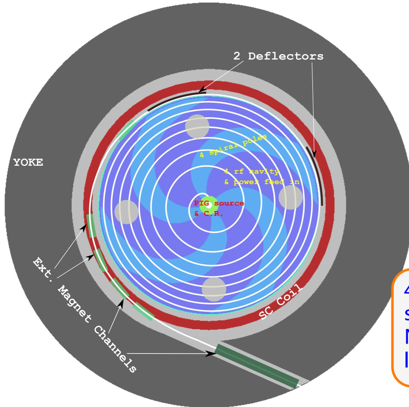
1) Internal cold cathode PIG source, simplification of injection, for moderate intensity  $\sim 500\text{nA}$
