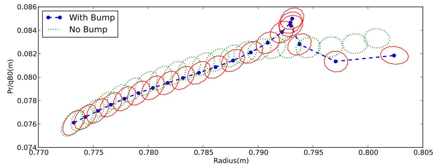
$b_1=6\text{Gs}$ ,  $\theta_0=30\text{ deg.}$ ,  $dR\sim 5\text{mm}$  (coincident with theoretical 4.3mm, eff. Turns = 9)
