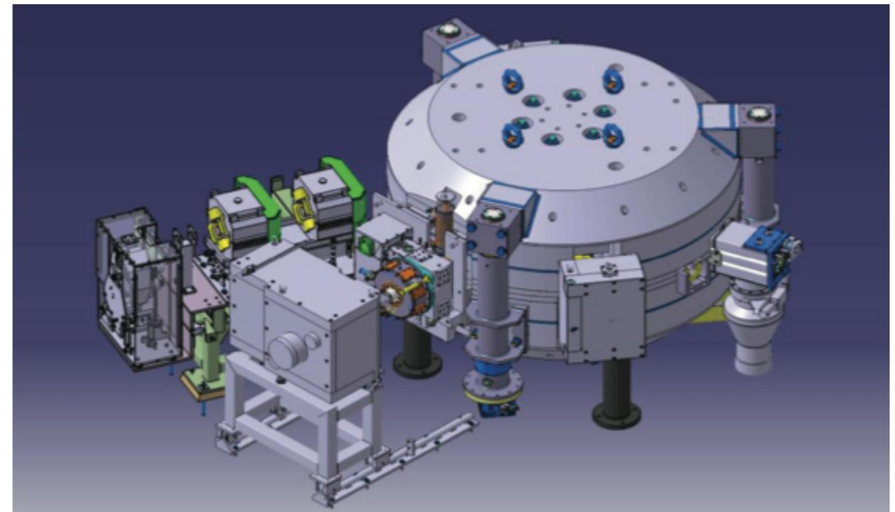
IBA S2C2 (superconducting synchro-cyclotron): max. 5.7T@C.R., 2.5m diameter, internal cold cathode PIG; 1k Hz rotco RF
