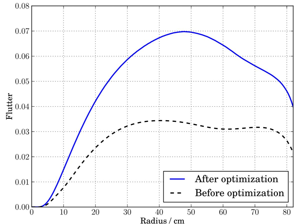
Enhanced field flutter by optimizing the magnet structure
