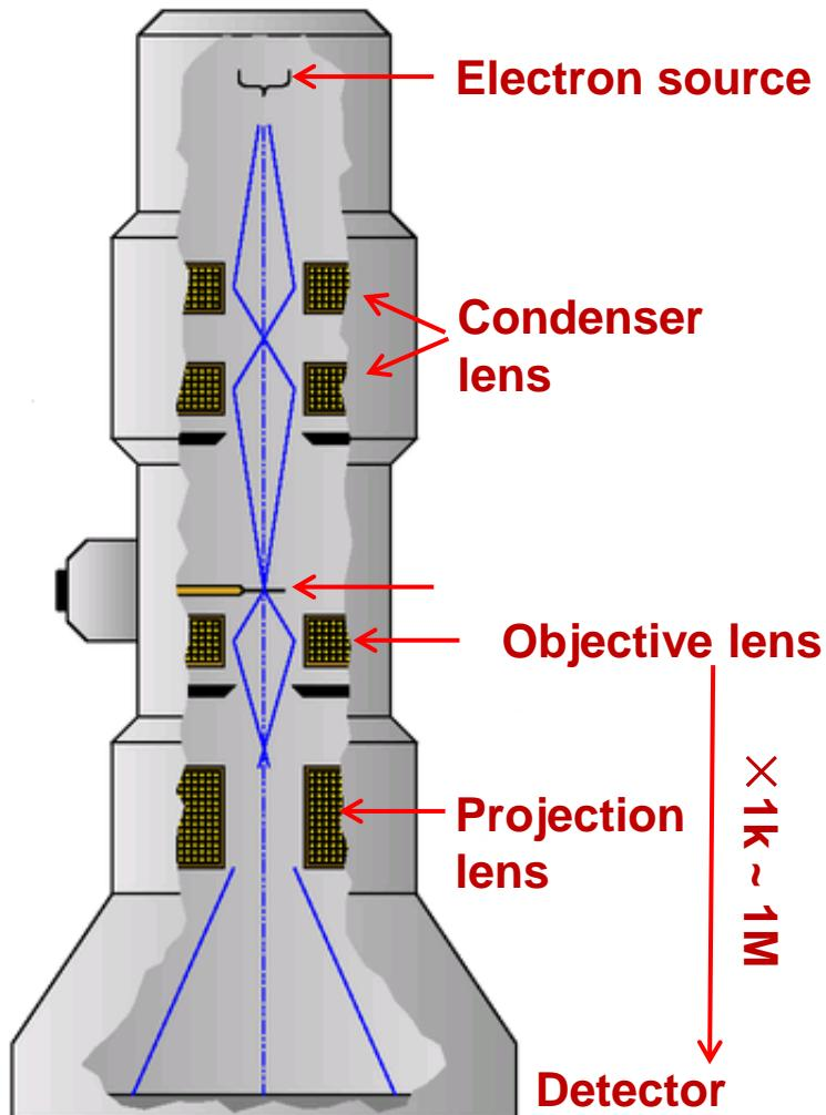
Schematic of a transmission electron microscope
