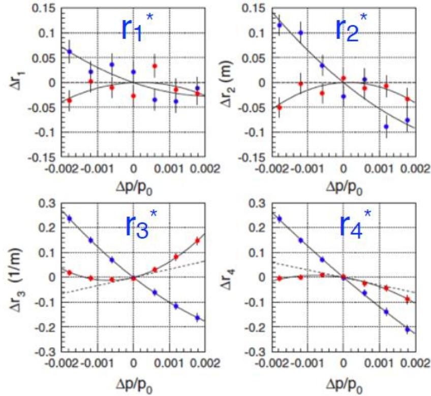
FIG. 4. (Color) Measured chromatic X-Y coupling at IP in LER. The blue plots indicate those before and the red plots indicate those after the skew sextupole correction. The dashed line indicates the natural chromatic X-Y coupling estimated using the model lattice by SAD.
