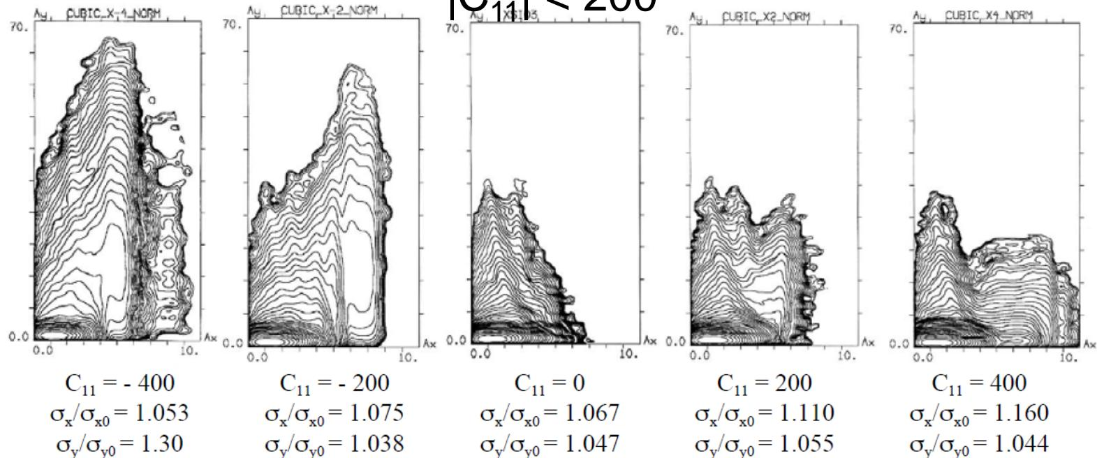
Figure 3. Beam-beam blow up and tail growth as a function of the cubic lattice nonlinearity (numerical simulations). Equilibrium density contour plots in the space of normalised betatron amplitudes are shown.
