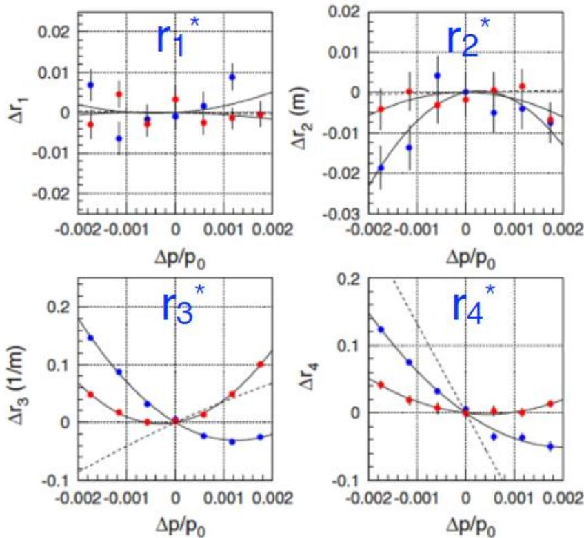
FIG. 3. (Color) Measured chromatic X-Y coupling at IP in HER. The blue plots indicate those before and the red plots indicate those after the skew sextupole correction. The dashed line indicates the natural chromatic X-Y coupling estimated using the model lattice by SAD.
