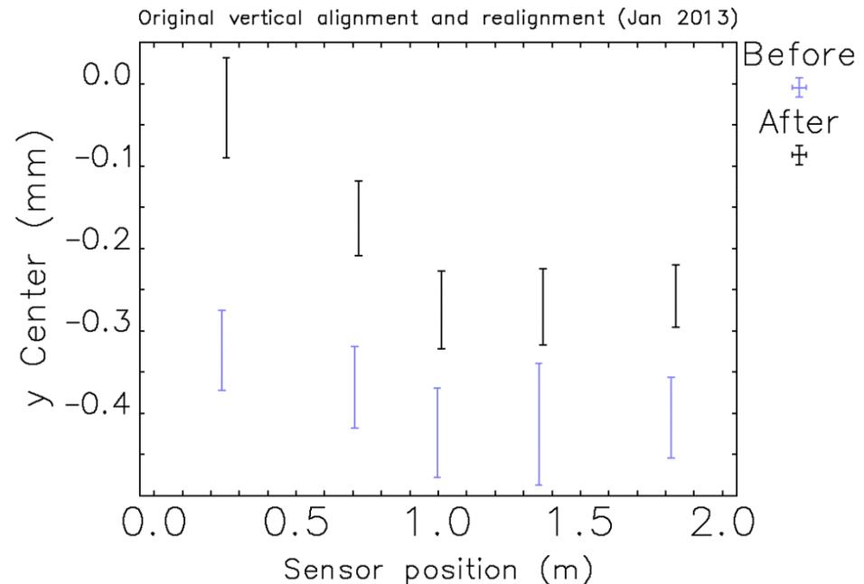
Vertical center of chamber with respect to the user beam orbit. Sensors 2-6, January 2013 data.
