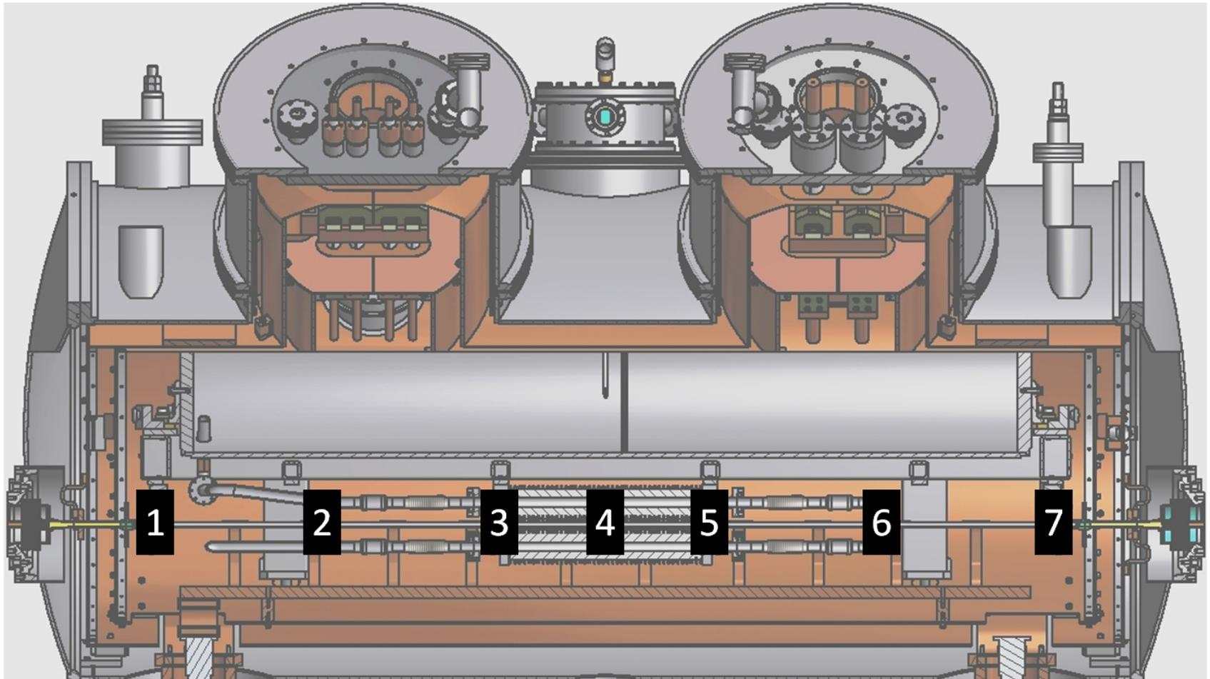
Positions 1, 3, 5, and 7 are at the beam chamber support locations.
