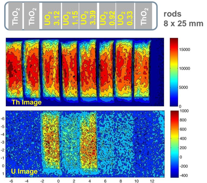
Uranium and Thorium fluorescence maps of mock fuel pellets encased in Zirconium.
