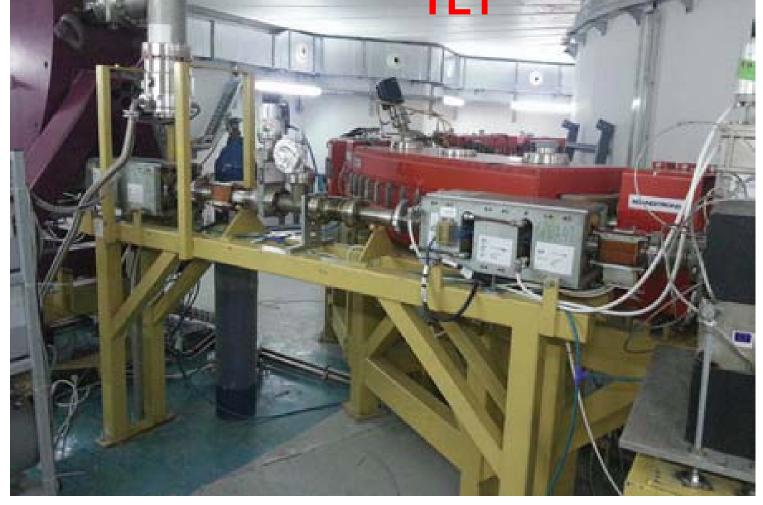
Booster Magnets are Installed and Aligned, Measurement uncertainty: ±0.05mm, 1 sigma for X and Z axis, ±0.15mm, 1 sigma for S axis and ±0.05mrad 1 sigma for Tilt. The Microtron and TL2 have been set up to their theoretical position.
