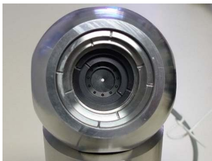
Fig. 10 Iris diaphragm target which can be opened to 12mm caliber with a remote controller.
