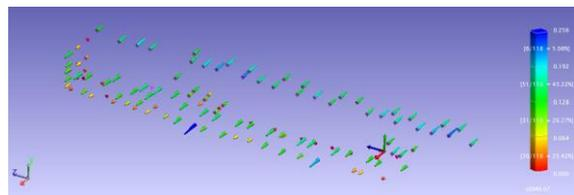
**Figure 14.** Deviation along X axis between the old and the new USMN network.
