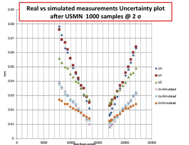
**Figure 7.** Comparison between the uncertainty of the simulations and the real survey on an almost straight line on the floor aligned with the beam line.
