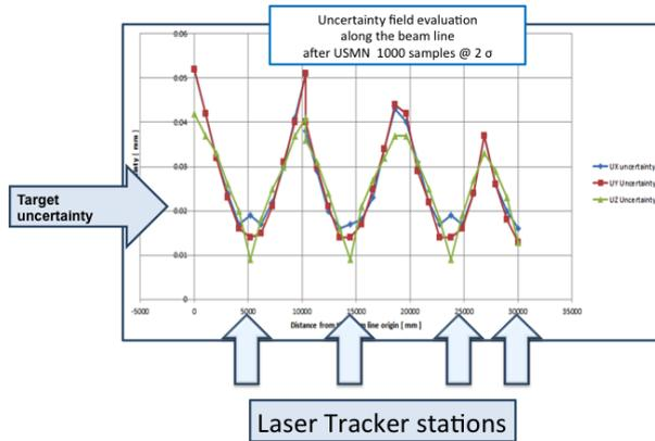
**Figure 5.** Result of SA simulations of measuring points on the floor aligned with the beam line from 5 tracker locations.
