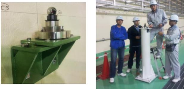
**Figure 11.** The references for the Taylor Hobson for the alignment of the injector: wall bracket on the wall (left) and the reference pillar (right).
