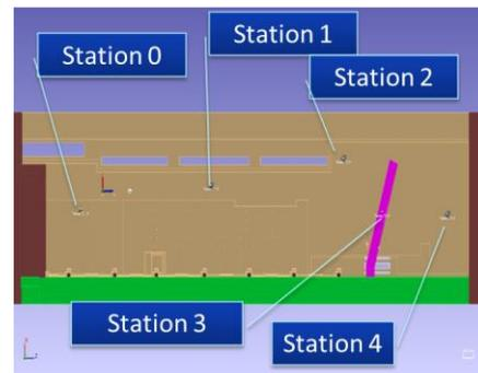
**Figure 2.** Position of each tracker station inside the accelerator vault
