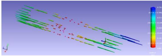
**Figure 16.** Deviation along Z axis between the old and the new USMN network.
