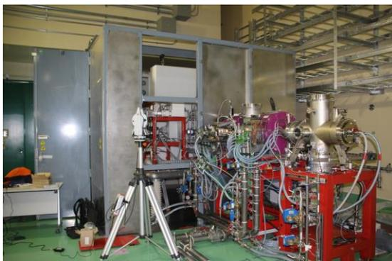
**Figure 12.** LEBT and source survey with the AT401 in the accelerator hall.
