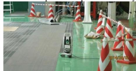
**Figure 10.** The tracker placed on the floor in order to increase accuracy reducing the influence of the angular encoder on the measurement.
