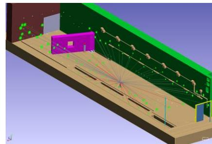
**Figure 3.** Typical network survey: all the visible network fiducials are measured to increase rigidity on the USMN algorithm to lower uncertainties.
