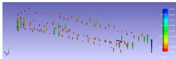
**Figure 15.** Deviation along Y axis between the old and the new USMN network.
