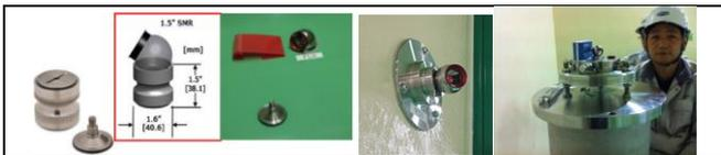
**Figure 6.** Floor nests (left), walls nest supports (center) and the datum pillar (right) installed in the accelerator vault.
