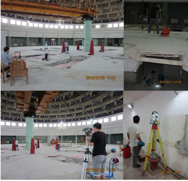
Fig.6: Actual measurement of the primary control network
