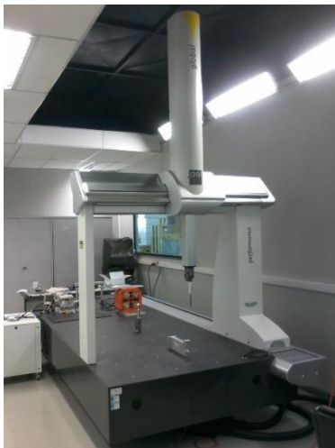
Figure 5: CMM from Hexagon Metrology™ used to perform the experiment.
