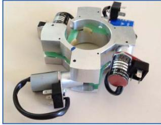
Figure 5: wire displacement system based on thermo-electrical motors
