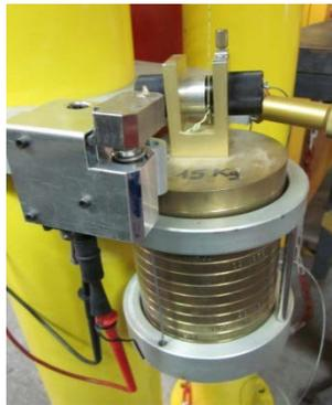
Figure 7: Wire break sensor
