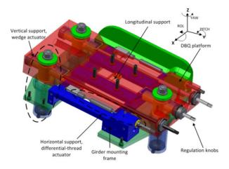
Figure 3: 3D model of 5 DOF adjustment system
