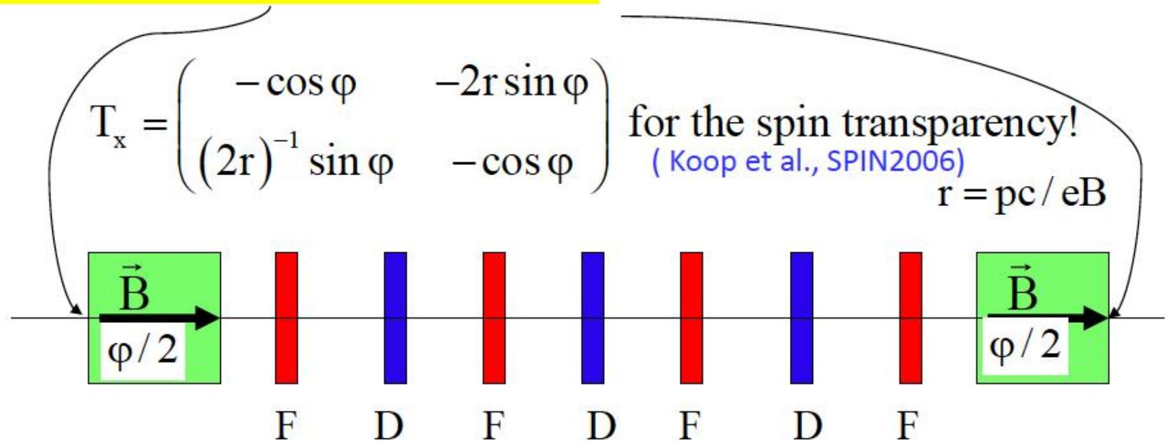
Two solenoids, each  $L=40$  m  $B=5$  T, provide spin rotation by  $\varphi = 180^\circ$  at  $E=45.5$  GeV. Extension to 120 GeV with  $B=10$  T looks feasible.
