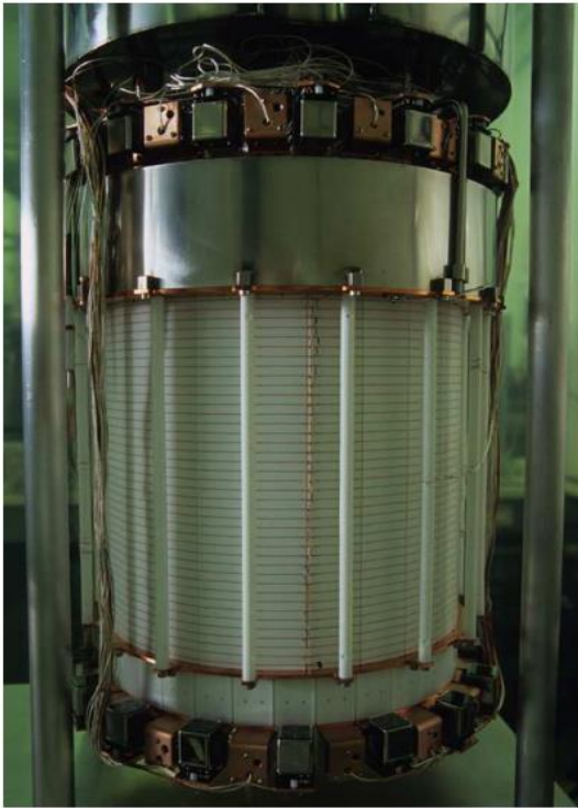
XENON100, 60 kg, completed 2012, Gran Sasso XENON1T in preparation
