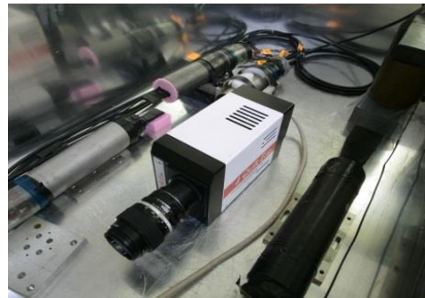
ICCD system and cosmic ray counter
