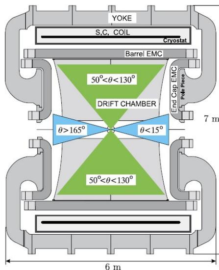
Fig. 1. Vertical cross section of the KLOE detector, showing the small and large angle regions where respectively photons and pions (or muons) are accepted.
