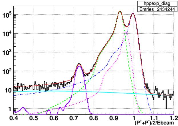
Fig. 5. Average momentum distribution for events with  $|\Delta P|/E_{beam} < 0.038$ ,  $E_{beam} = 391.48\text{MeV}$ , where histogram - data, lines - projection of fitted functions after minimization: the peaks from left to right  $3\pi$ ,  $2\pi$ ,  $2\mu$ ,  $e^+e^-$ , cyan line - cosmic events
