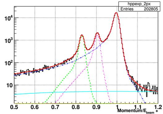
Fig. 4. Momentum distribution of positive charge particles for  $E_{beam} = 252.8$  MeV, where histogram - data, lines - projection of fitted functions after minimization: the peaks from left to right -  $\pi^+$ ,  $\mu^+$ ,  $e^+$ , cyan line - cosmic events
