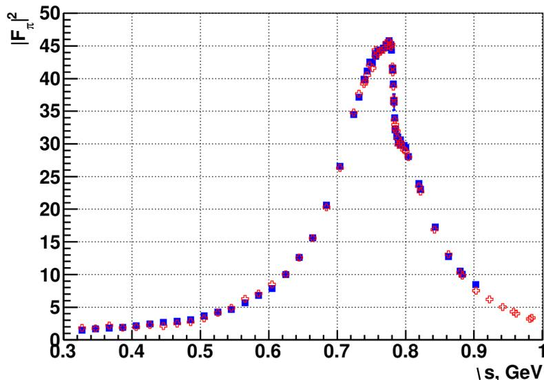
Fig. 8. Preliminary results on  $F_\pi^2$  from CMD-3. Open crosses – separation done on the calorimeter information, filled squares – on particle momentum. Some additional corrections, common to two methods (e.g., the trigger efficiency), are not applied
