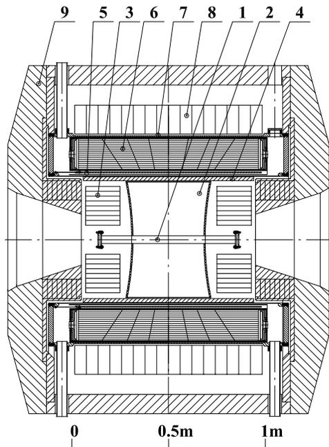
Fig. 1. CMD-3 detector: 1 – beam pipe, 2 – drift chamber, 3 – BGO calorimeter, 4 – Z-chamber, 5 – SC solenoid (0.13 $X_0$ , 13kGs), 6 – LXe calorimeter, 7 – TOF system, 8 – CsI electromagnetic calorimeter, 9 – yoke, not shown muon range system
