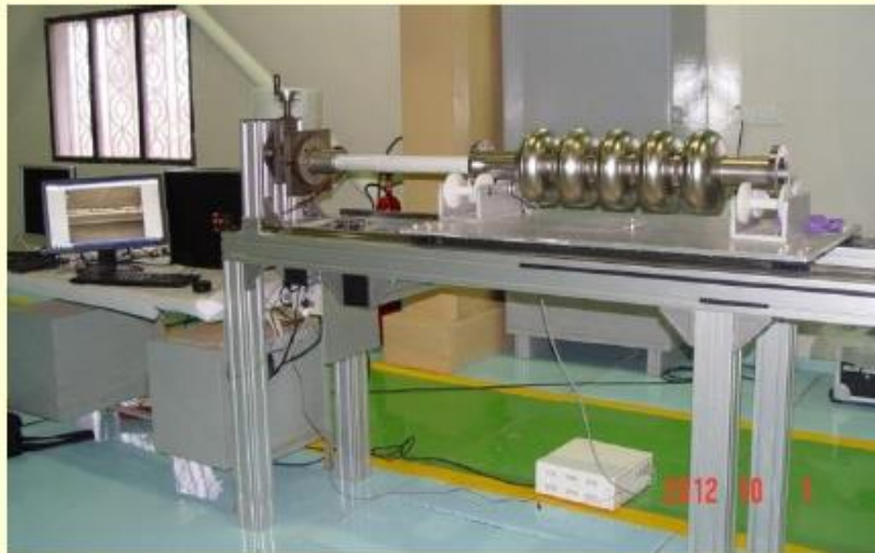
Optical inspection bench for multi-cell SCRF cavities
