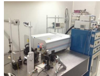
2K system, LLRF control, 20kW solid state RF amplifier, and drive laser
