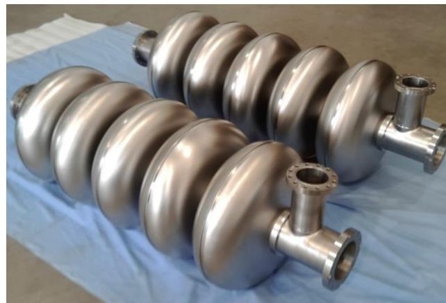
650 MHz \beta=0.82 5-cell cavity vertical test soon
