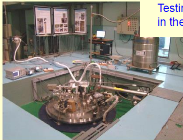
Transfer of liquid helium in the VTS cryostat
