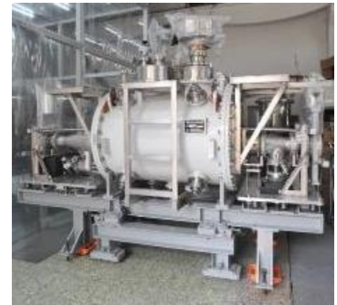
500 MHz cavity module horizontal tested
