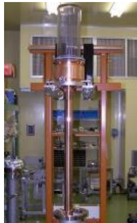
500 MHz coupler 420 kW CW TW
