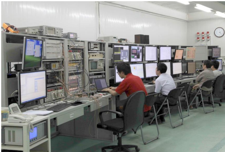
2K system, LLRF control, 20kW solid state RF amplifier, and drive laser
