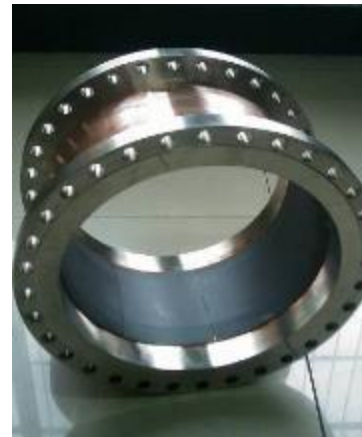
HOM absorber ferrite 6kW
