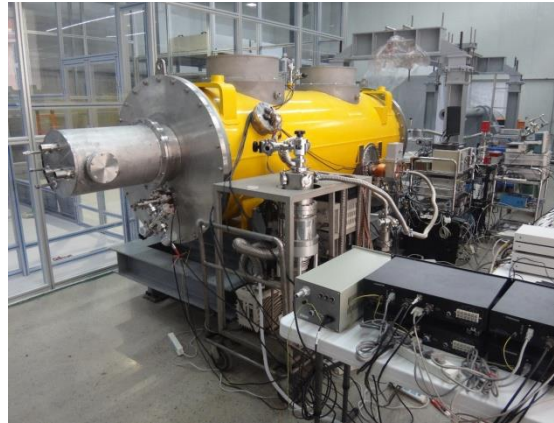
1.3 GHz test cryomodule horizontal test soon
