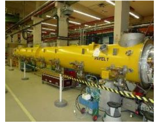
12 m 1.3 GHz cryomodule for Euro-XFEL
