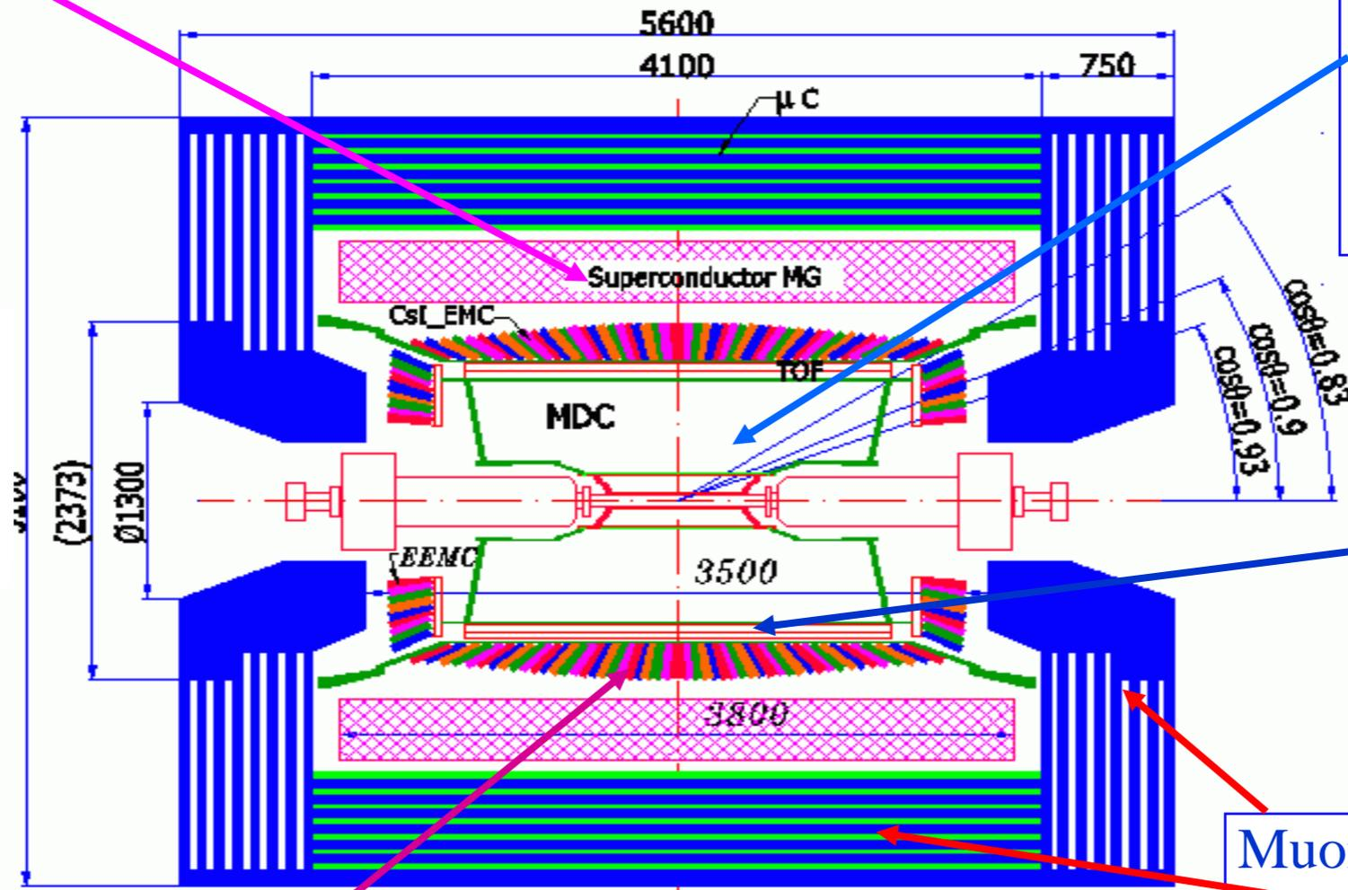
hermetic spectrometer for neutral and charged particle with excellent resolution, PID, and large coverage.
