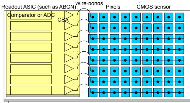
• We will contribute to the sensor design and test. Design contribution being discussed; prototype sensors for test on the way.
