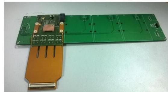
APV25 with the new FPC connector, mounted on a backplane
