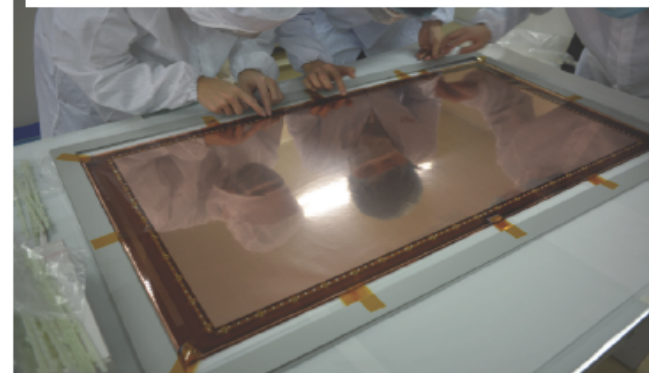
Placing the second GEM foil
