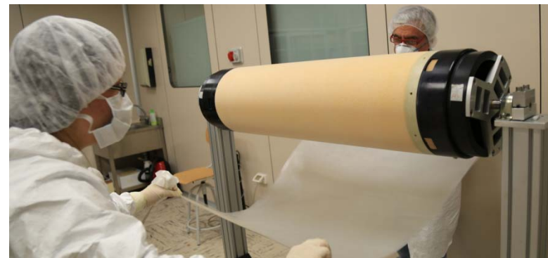
Rohacell plane is glued on the kapton.
