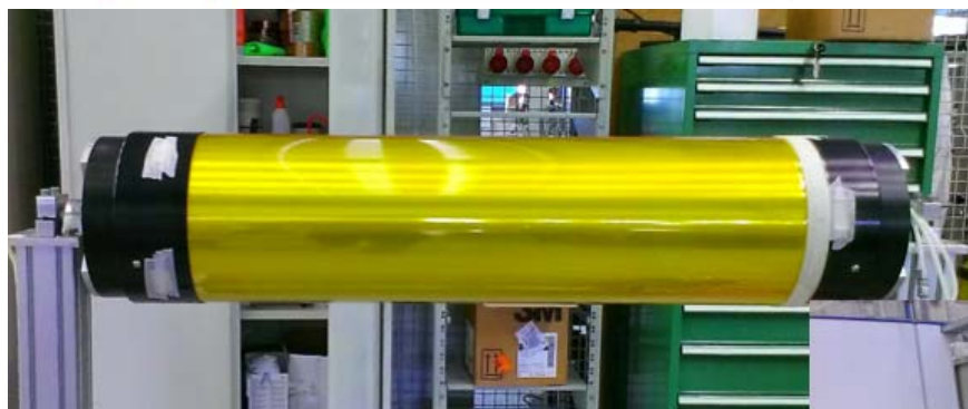
12.5 \mu\text{m} kapton foil around the Al mold;
