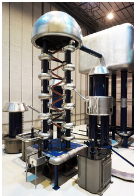
The PSI Cockcroft-Walton accelerator – the first stage of the proton accelerator facility.
