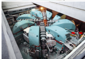
The magnets are coloured turquoise and the four acceleration cavities dark grey.
