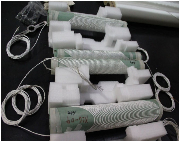
Finished winding, to be vacuum impregnated and assembled
