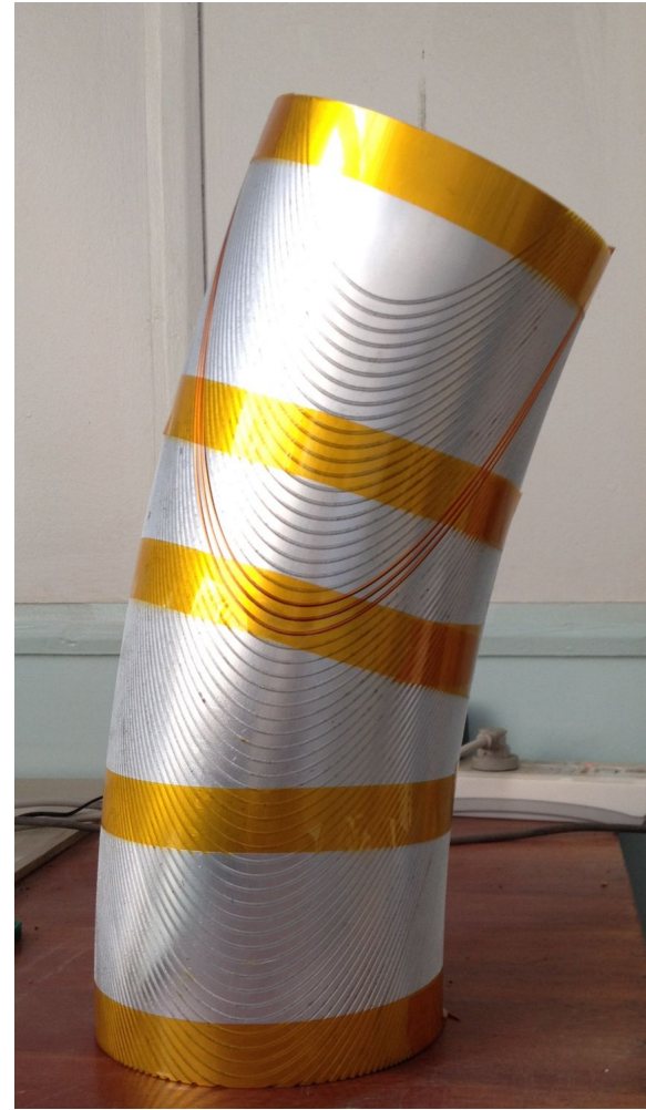
Sample mechined with CNC grinder
