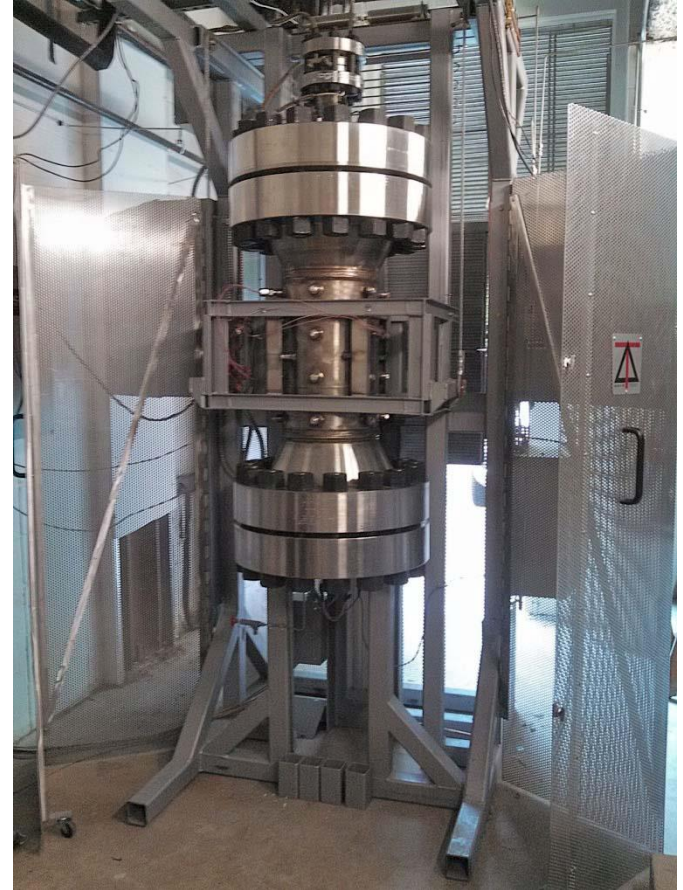
Our 100 bar 900 °C furnace with 14 cm dia. X 50 cm long hot zone
