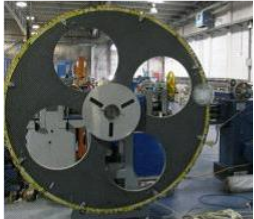
Coils for 220 kV HTS Fault Current Limiter
