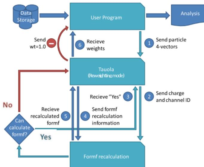
**Figure 2:** Flow chart for communication when already stored events are modified with the weights.
