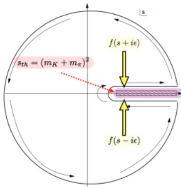
$$F_+^{\pi^- \eta^{(\prime)}}(s) = \frac{1}{\pi} \int_{s_{th}}^{\infty} ds' \frac{\text{Im} F_+^{\pi^- \eta^{(\prime)}}(s')}{s' - s - i\epsilon}$$
