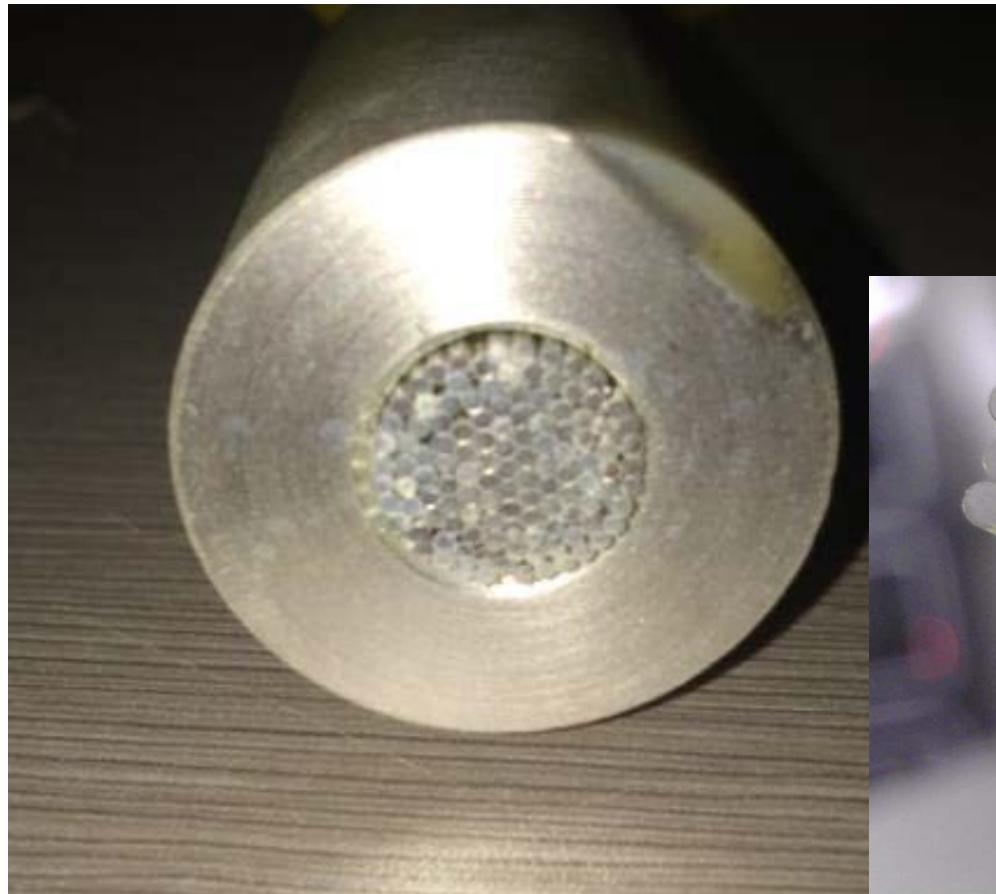
The end of fiber is plated with silver, but the edge of plating mirror is easily peeled off
