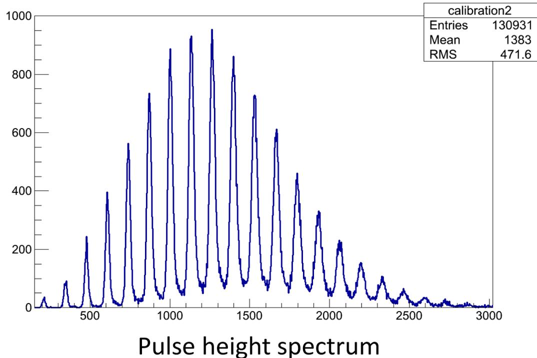
The individual peaks are clearly separated from each other in the pulse height spectrum.
