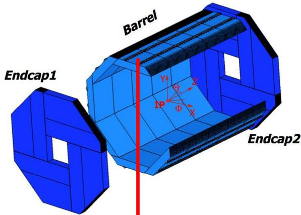
The CEPC ECAL consists of a cylindrical barrel system and two end caps.
