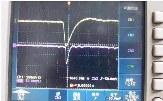
Waveform of strip counter and trigger counter
