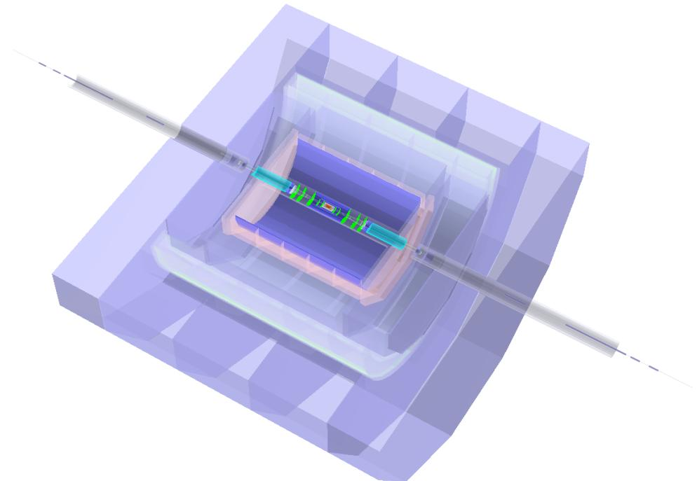
A detector reconstructs all the physics objects (lepton, photon, tau, Jet, MET, ...) with high efficiency/precision
