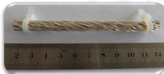
Bi2212 strands cabling and CICC structure
