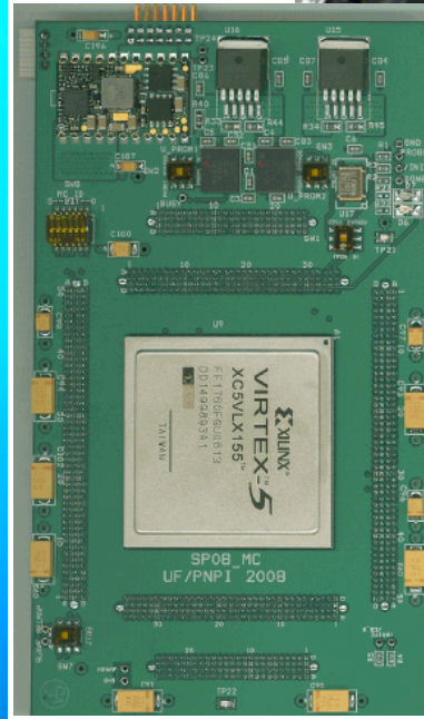
CSCTF transition board and connection cables to DTTF with Channel-Link LVDS transmission
