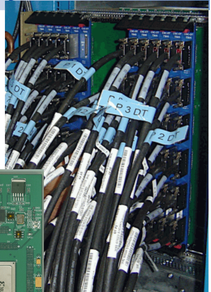
CSCTF transition board and connection cables to DTTF with Channel-Link LVDS transmission
