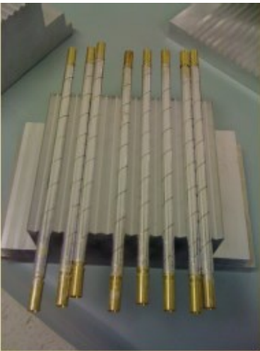
Doublet of UV straw chambers
