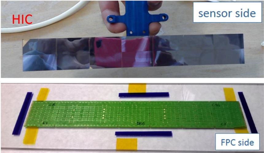
HIC (Hybrid Integrated Circuit) module: FPC + 2X7 pixel chips (Outer) or FPC + 1X9 pixel chips (Inner)
