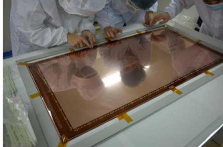
GEM assembly using a novel self-stretching technique
