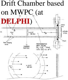
Fig. 5. Principle of a slow RICH detector using electron drift over long distances.
