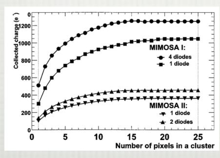
AMS 0.6 µm technology - 14 µm epitaxial layer - 20 µm pixel pitch
