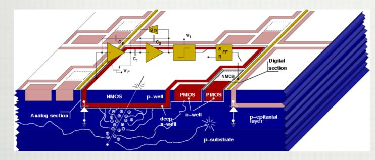
In triple-well CMOS processes a deep N-well is used to isolate N-channel MOSFETs from substrate
