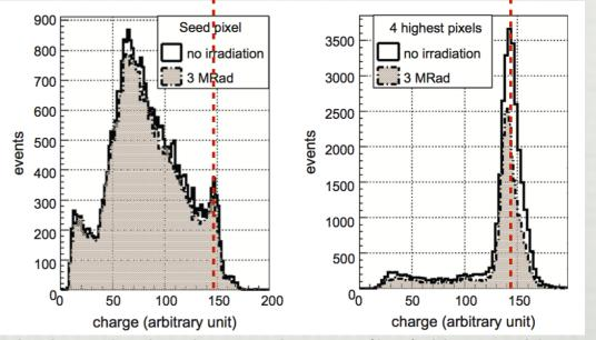
TJ 0.18 µm technology - 18 µm epitaxial layer - 20 µm pixel pitch, illuminated by an 55fe source (5.9 keV X ray, 1640 eh pairs b.shorter collection time ---> reduced trapping probability ---> increased radiation tolerance (possibly from 10<sup>12</sup> n<sub>eq</sub>/cm<sup>2</sup> to 10<sup>15</sup> n<sub>eq</sub>/cm<sup>2</sup> [W. Snoeys, NIM A731 (2013) 125]
