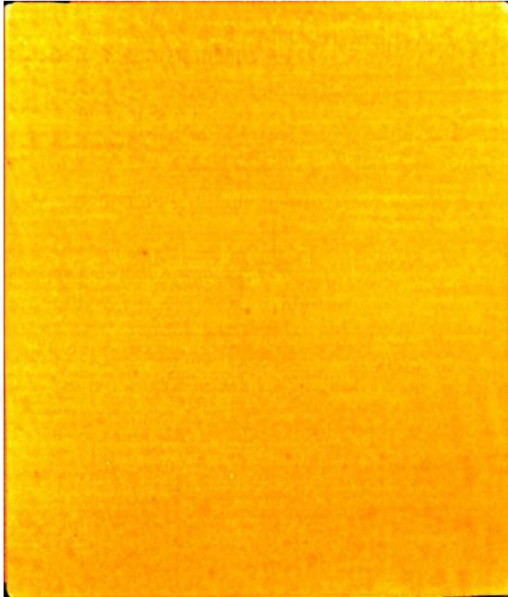
Gain map image for a pair of 20 \mu\text{m} pore, 60:1 L/D, ALD borosilicate MCPs, 950 V per MCP, 184 nm UV
