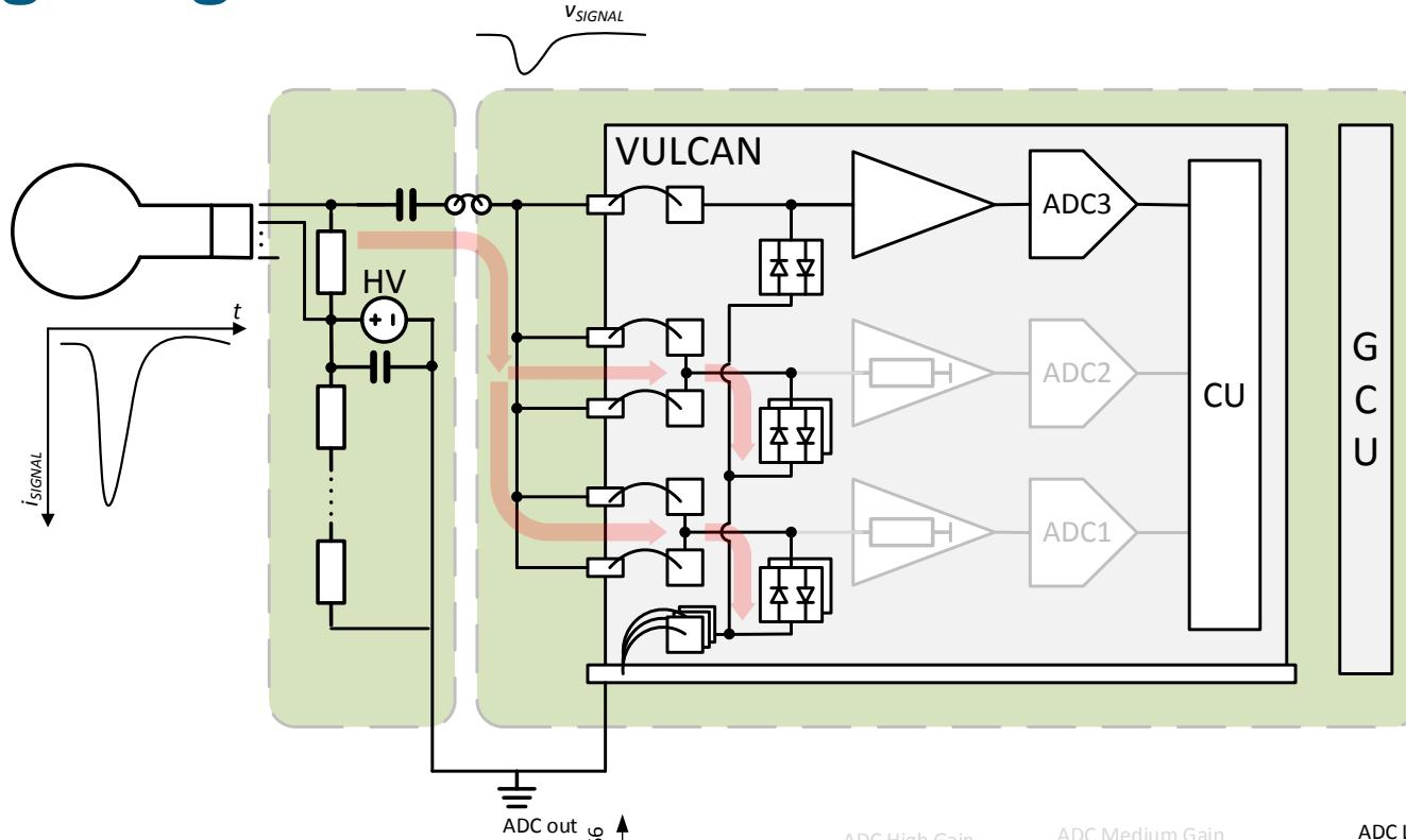
With larger input currents  $>20\text{mA}$  the TIA inputs saturate, the ESD diodes open with a combined resistance  $R \approx 5\Omega$ , The voltage over the diodes is measured with the third signal chain
