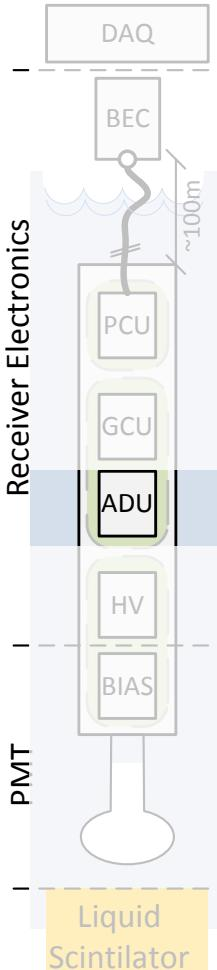
1. Approx. 80dB linearity by using 3 signal chains for 3 different signal ranges
