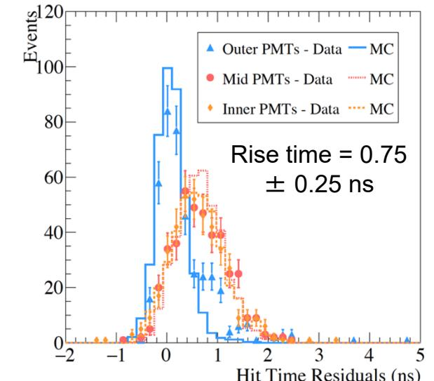
Full simulation includes detailed geometry, DAQ effects (TTS, pulse shapes, electronics noise...)
