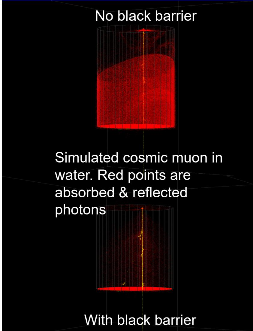
Simulated cosmic muon in water. Red points are absorbed & reflected photons
