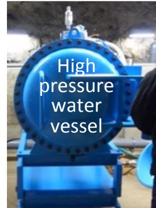
A set of the cover packed in a plastic bag was pressurized from outside. Tested two samples to 1.1MPa (=100 m water depth) and there were no damages. → OK for 100 m water load
