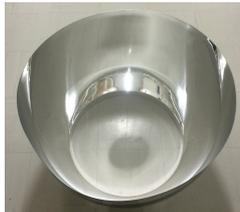
Winston cone for 20" PMT made of PET+Al
