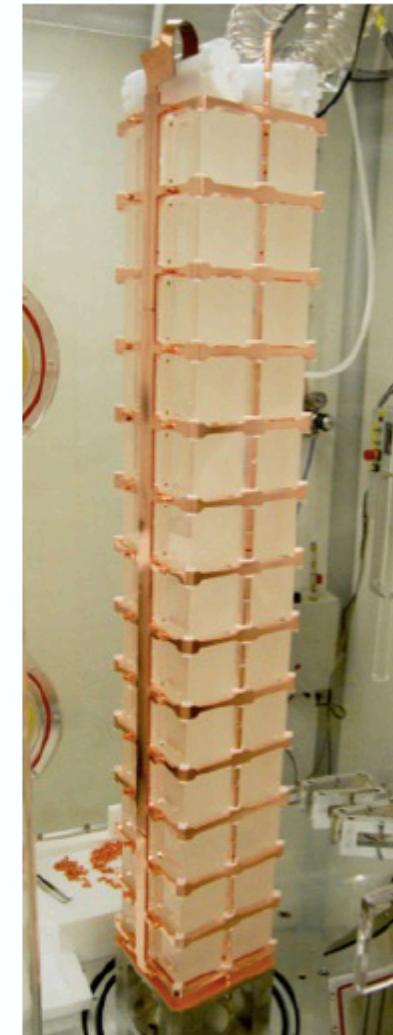
Operated in former Cuoricino cryostat, with improved energy resolution, background level (materials selection, cleaning and handling), duty cycle and detector response model
