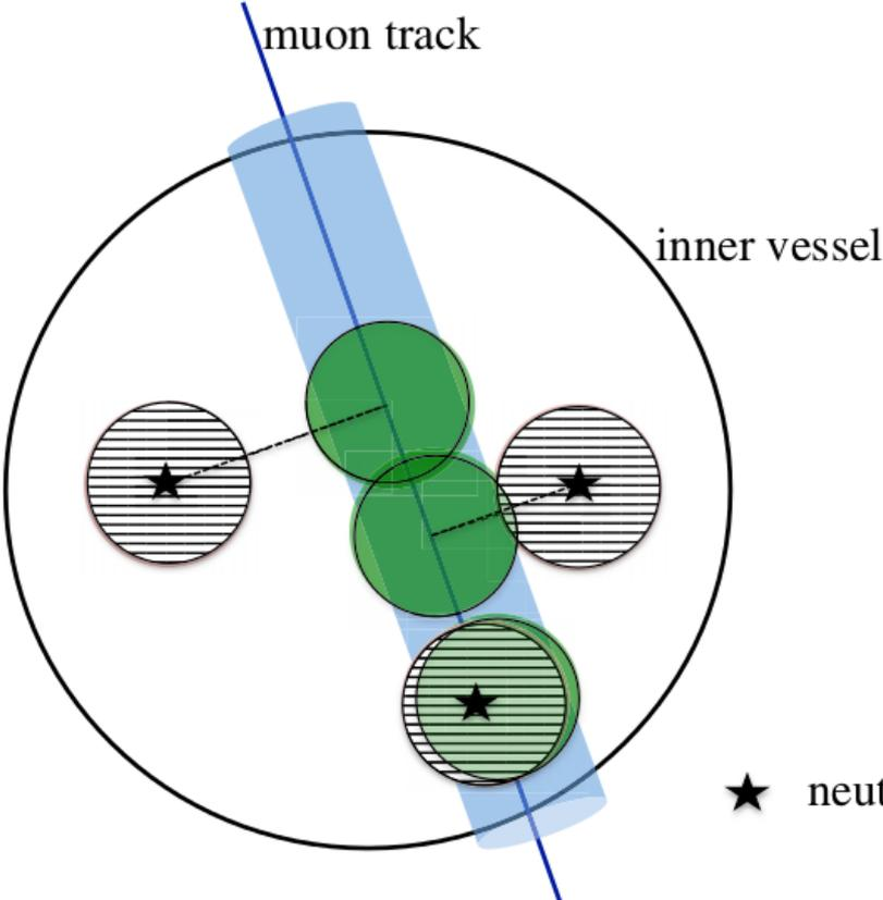
The diagram illustrates the Borexino detector setup. A blue line labeled "muon track" passes through a blue shaded region representing the muon track. The track enters a large circle labeled "inner vessel". Inside the vessel, three green circles represent neutron capture events, each marked with a black star. Dashed lines connect these stars to a legend at the bottom right: "★ neutron capture".
