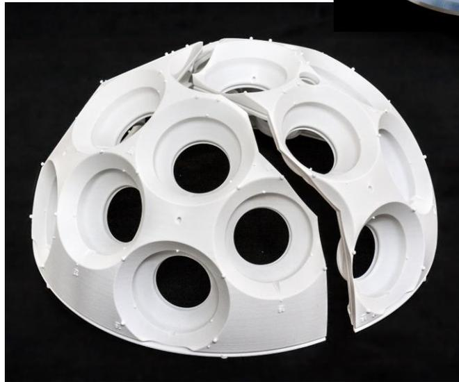
3D printed support structure (SLS)
