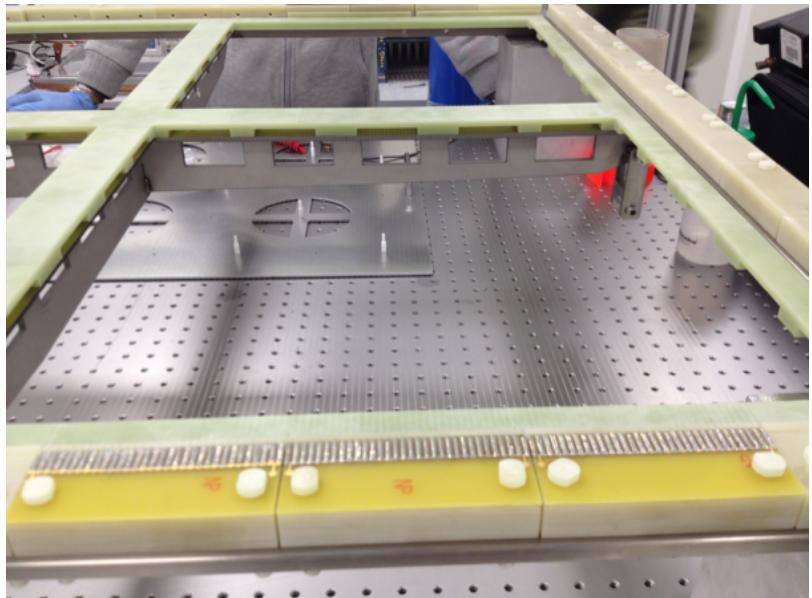
Wire soldering PCB and extraction grid
