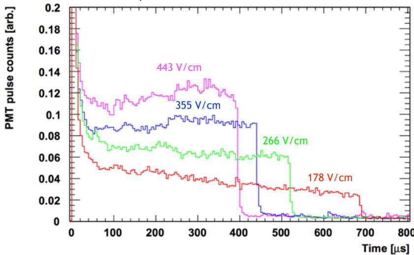
Drift velocity vs.  $E_{\text{drift}}$ :
