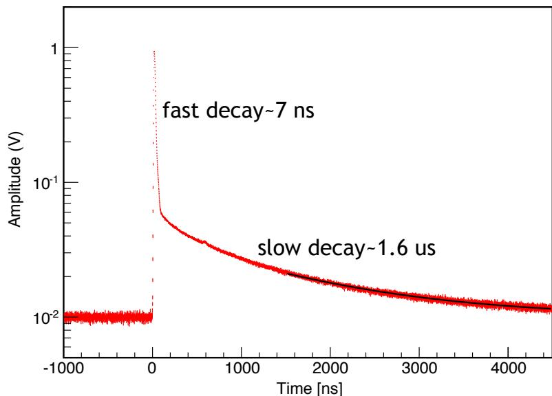
PMT coated with wavelength shifter TPB:
