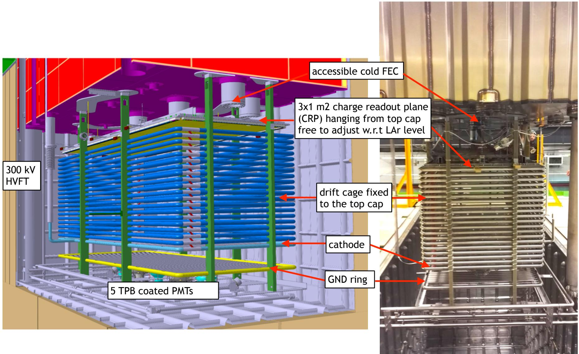
The 3x1 m<sup>2</sup> CRP
