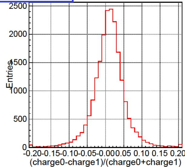
Uniform response to track azimuth angles:
