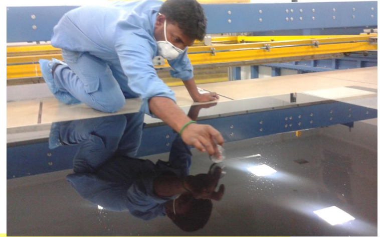
Production of 2mx2m glass RPC gap at Saint Gobain industry
