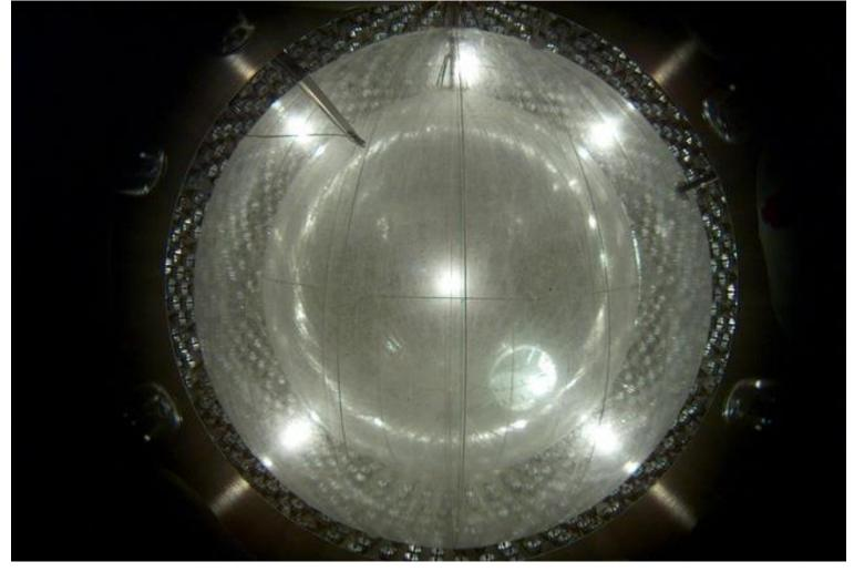
The nylon vessels were inflated in the sphere with synthetic air:  $C_{Rn} < 100 \mu Bq/m^3$
