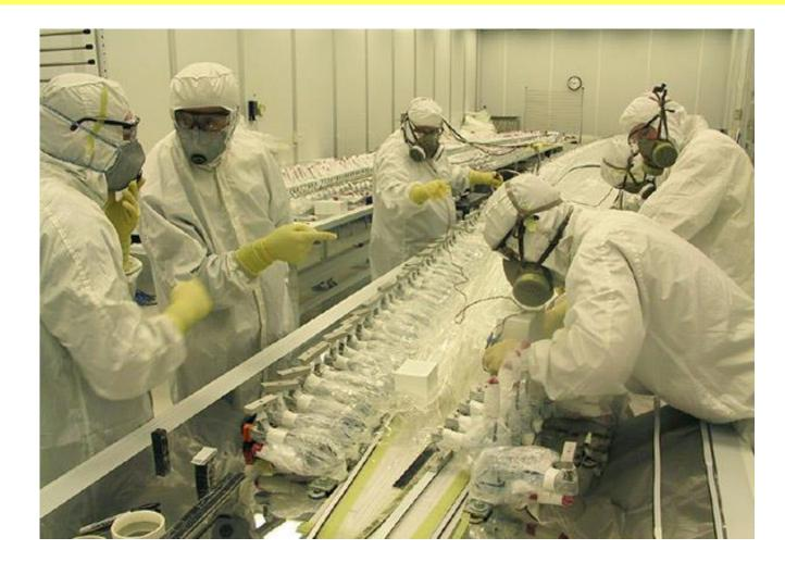
Princeton clean room class 100 with  $^{222}$ Rn-reduced air (VSA filter):  $C_{Rn} \sim 1 \text{ Bq/m}^3$
