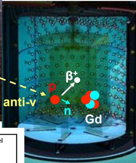
The anti- $\nu_e$  are detected **via inverse  $\beta$ -decay (IBD) reaction:**
