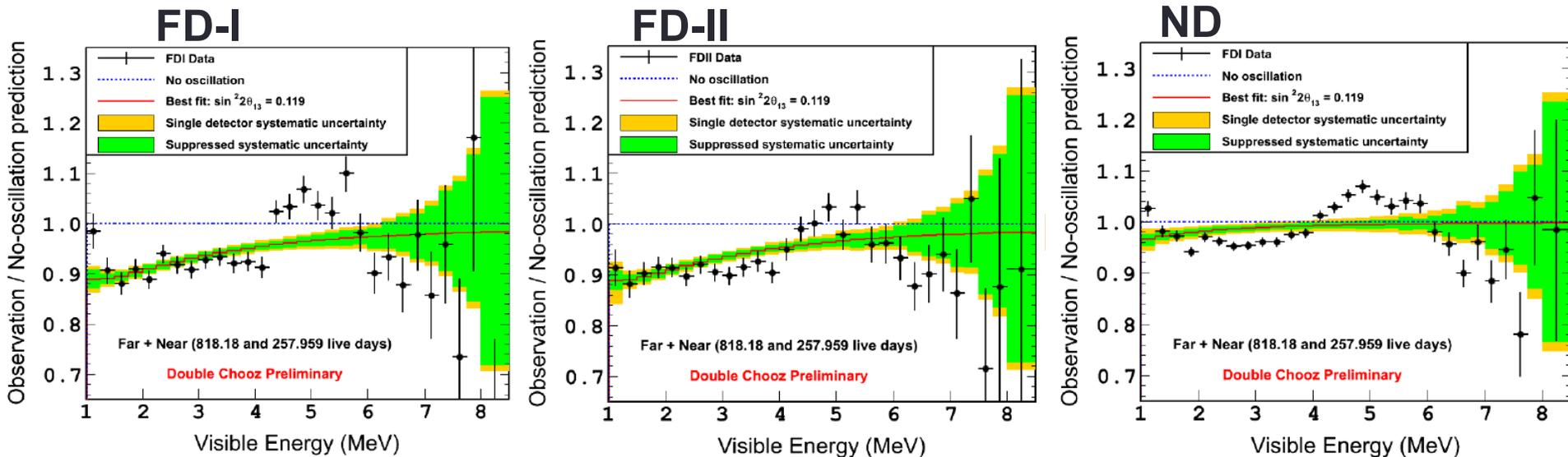
$$\sin^2(2\theta_{13}) = 0.119 \pm 0.016 \quad (\text{stat.} + \text{syst.}) \quad (\chi^2/\text{dof} = 236.2/114)$$
