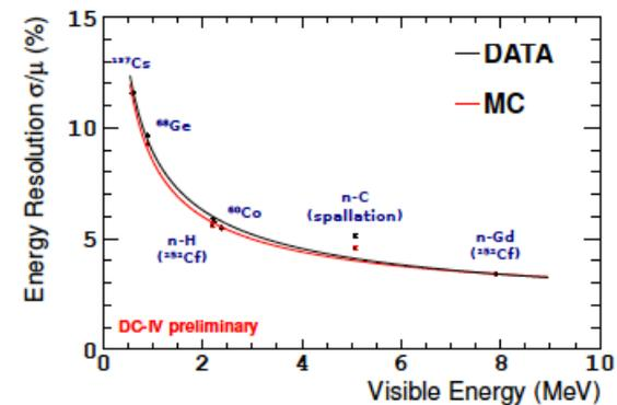
$$\sigma/E_{vis} = \sqrt{\frac{a^2}{E_{vis}} + b^2 + \frac{c^2}{E_{vis}^2}}$$
